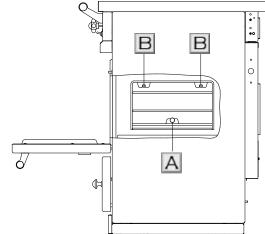
After cleaning, replace the back panel with the screws and the washers. Be sure you the screws are correctly screwed.
